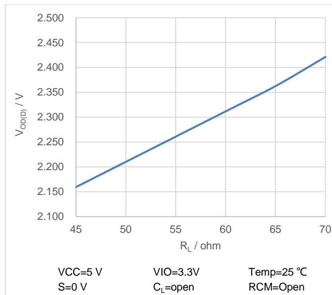
Figure 6-9  $V_{OD(D)}$  vs  $R_L$
