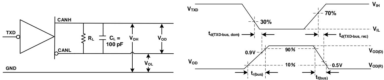
Figure 6-1 Driver Test Circuit and Voltage Waveforms
