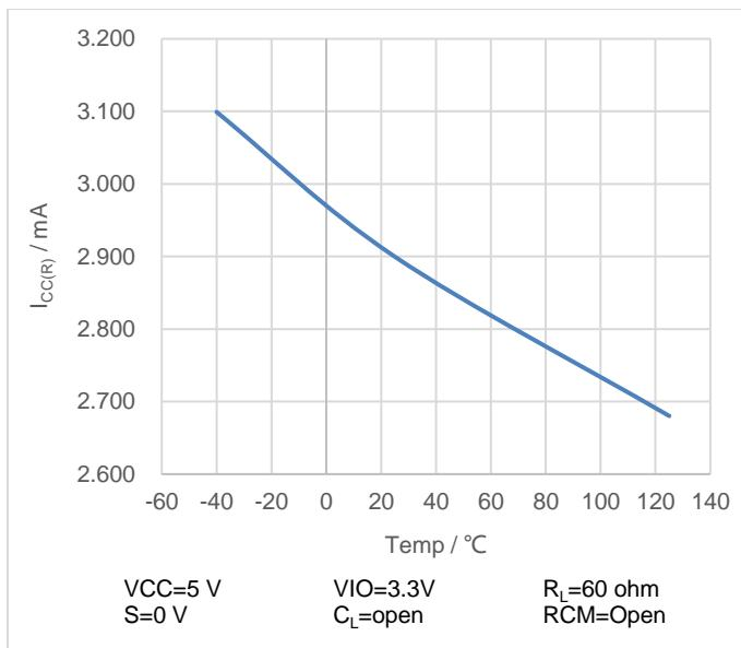
Figure 6-11  $I_{CC(R)}$  vs Temperature
