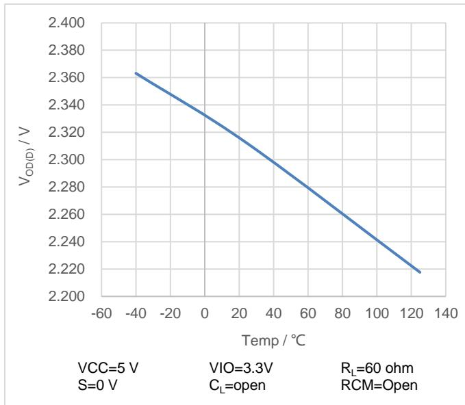
Figure 6-10  $V_{OD(D)}$  vs Temperature
