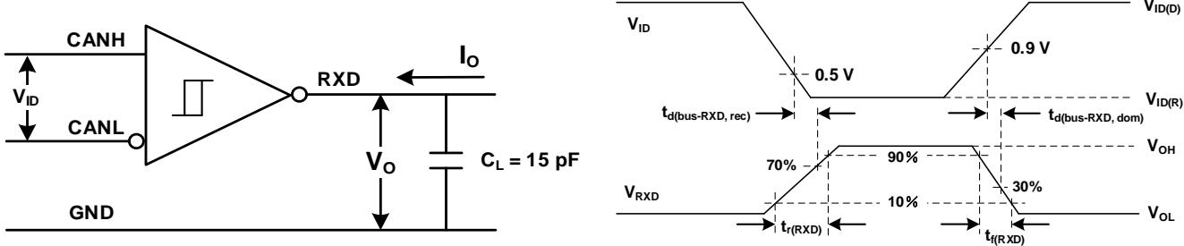
Figure 6-2 Receiver Test Circuit and Voltage Waveforms
