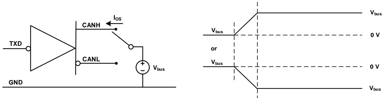
Figure 6-6 Driver Short-Circuit Current Test Circuit and Waveforms
