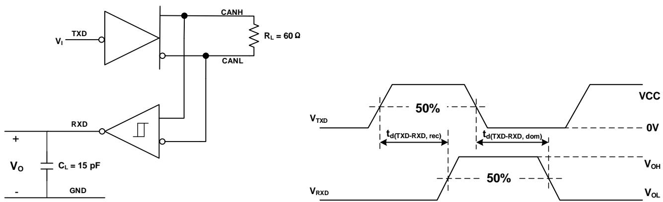
Figure 6-4 Loop Time Test Circuit and Voltage Waveforms
