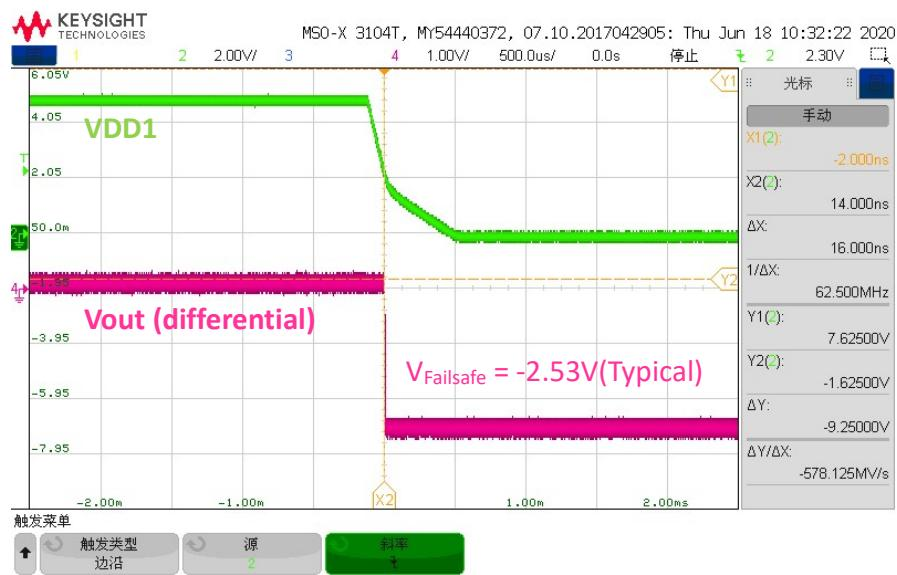
Figure 7.3 Typical Failsafe output when VDD1 undervoltage
